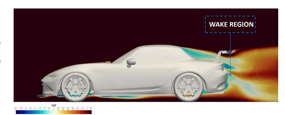
The CpT Plot shown above is used to visualize the wake region behind the car. The blue zone behind the vehicle is the wake and minimizing this as much as possible will reduce drag.
