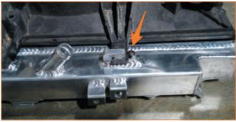
**17.** Thread the provided M4 Allen bolts into the upper fan shroud mounts and snug them down. Do not over tighten them.
