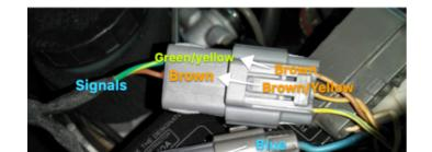
Note that in April 2020 we released the V2 NA6 patch with more intuitive wire colors. See the table below to identify the wiring of your version.
