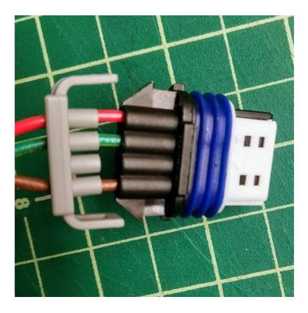
Start by removing the wire guard
