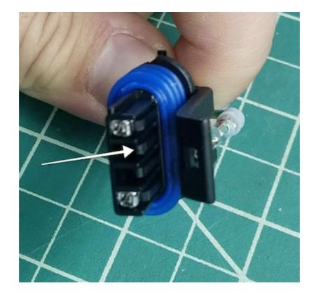
Use a small flat screwdriver or pick to pull up on the retainer clip, and pull out the middle wire.
