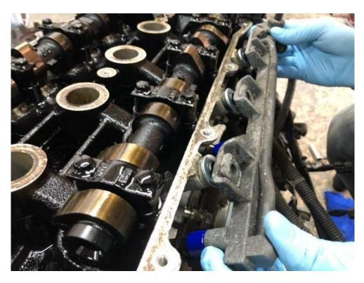
The injectors are based on the Bosch EV14 and have a V shaped spray pattern. For this reason they should be installed with the connector straight up or straight down wherever possible. In some cases, the shape of the Intake Manifold prevents perfect positioning, but try and get as close as you can.
