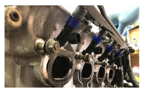
Use the original OEM bolts to secure the fuel rail, tighten each bolt bit by bit to push everything together evenly. There is no need to over tighten these, the OEM Torque Spec is 14-19 ft-lbs.
