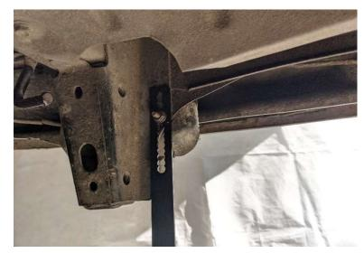
4) Secure the vertical brackets. Place the vertical bracket on the stud and reinstall the nut that was previously taken off. The bracket allows for adjustability for your car and preferences. For an NA (90-97) the 4<sup>th</sup> hole from the top works well as it gives the diffuser a 7degree angle which is good for downforce using this diffuser design. The bracket must also be pointing straight down and not at an angle.
