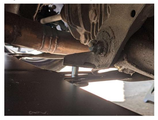
8) Bolt the diffuser to the vertical bracket. Use the supplied M8 bolts and nuts to secure the rear of the diffuser to the vertical bracket. Make sure to a washer on both sides of the diffuser as well as the lock nut.
